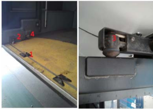
Figure 3. Components of the door system: 1-bottom track, 2-bottom guide, 3-door hinge with a potentiometer, 4-door arm tip
