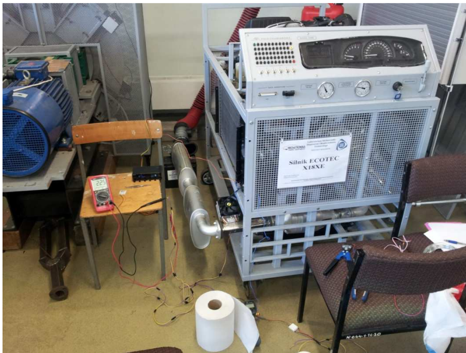
Fig. 1. Photo of the testbed with ECOTEC X18XE engine .
